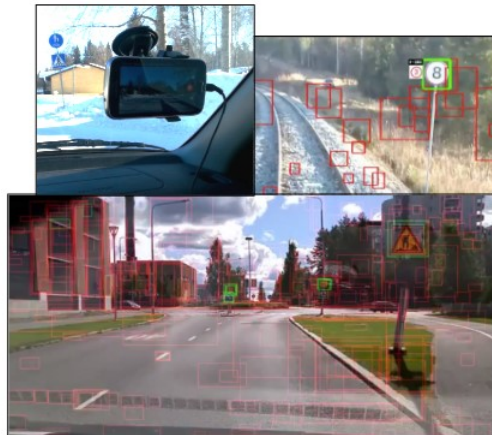
Low cost data collection, defect detection and automated inventorying
